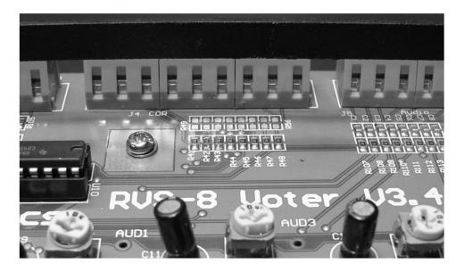
You will need eight, 4.7K ohm, 1/8 watt, wire lead, resistors. Cut each resistor so that one end has 1/4" of wire. Do not cut the other end yet.
