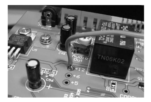
That completes the wiring. Turn on the voter and go to the Menu for COR Active State and select Lo for all channels.
