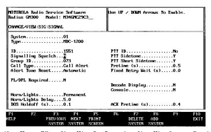
Figure 2-12. Changel View, Signalling Configuration, Signalling System, Receive Radio
