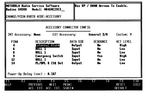
Figure 3-4. Change/View, Radio Wide, 16-Channel Receive Radio Accessory
