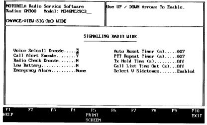
Figure 2-16. Change/View, Signalling, Radio Wide, Console Radio
