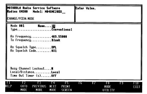
Figure 3-8. Change/View, 8-Channel Receive Radio Mode
