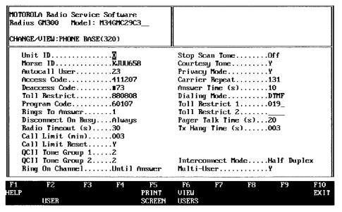
Figure 6-8. Setting System Wide Parameters
