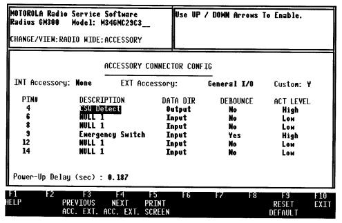
Figure 5-5. Change/View, Radio Wide, 16-Channel Transmit Radio Accessory
