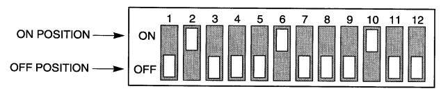
Figure 3-7. S2 Settings for Unidirectional Repeater Using an 8-Channel GM300, M10, or M120 Transmit Radio
