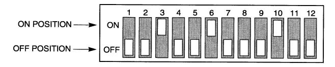
Figure 3-9. S2 Settings for Unidirectional Repeater Using an 8-Channel GM300, M10, or M120 Receive Radio
