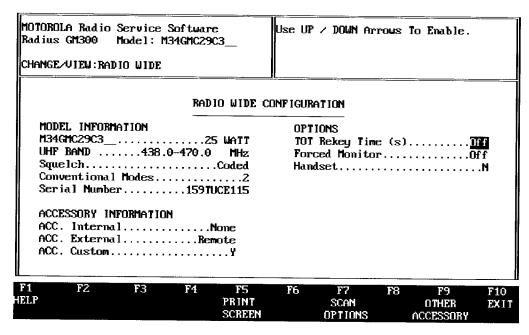
Figure 8-4. Change/View, Radio Wide, Transmit Radio
