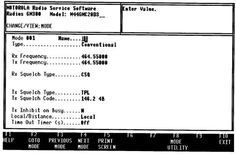
Figure 5-4. Change/View, 8-Channel Transmit Radio Mode
