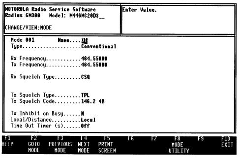
Figure 5-7. Change/View, 8-Channel Transmit Radio Mode
