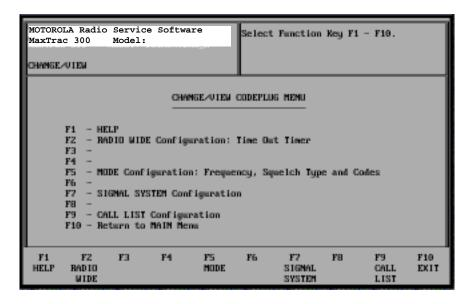
Function **F2** allows changes to the Time-Out Timer and the Scan Second Priority Channel. Function **F5** allows changes to the modes. These include Frequency, Squelch Type, PL/DPL codes and Mode Scan Lists (MaxTrac 300 only). Data fields may be edited as described in Part 1. Functions **F7** and **F9** are used for signaling radios and will be discussed in Part 4.
