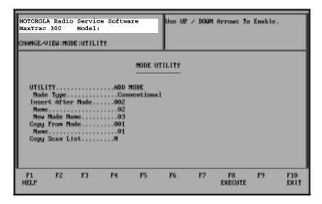
The Add Mode function allows you to add modes to the radio. Move Mode allows you to move mode information to a new mode number. Delete Mode allows you to delete modes from the radio. Copy Mode allows you to copy mode information from one mode to another. Each of these utilities is described below.
