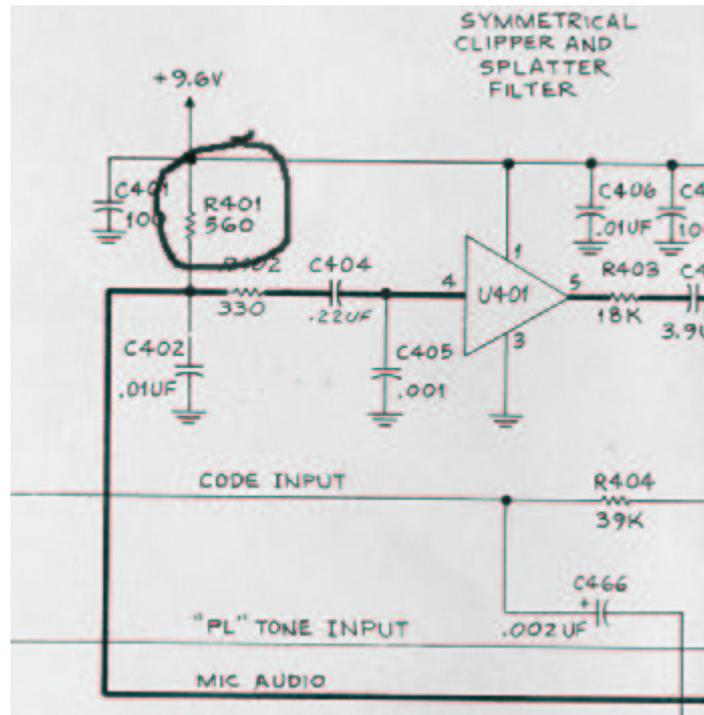
1.) See reference 1. Remove R401 to increase tx audio input impedance and to remove the dc bias from the mic audio line.. This is most likely a 560 ohm resistor. On the board in my base station, this resistor had already been removed.
