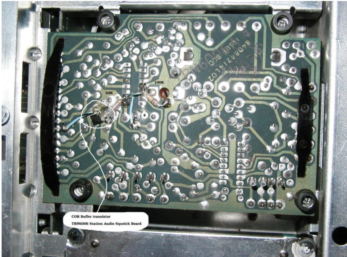
Steps 4-11 convert the station version of the audio/squelch board (TRN-6006A) to be more useful for ham controller use. See reference 5 for detailed instructions. The meat of the conversion is replicated here.
