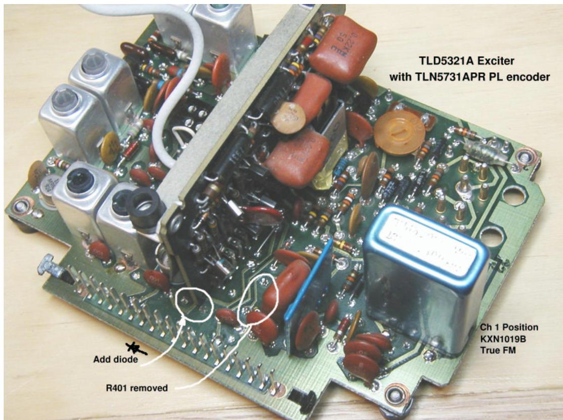
2). There are two options of modification to allow proper keying of the exciter if
