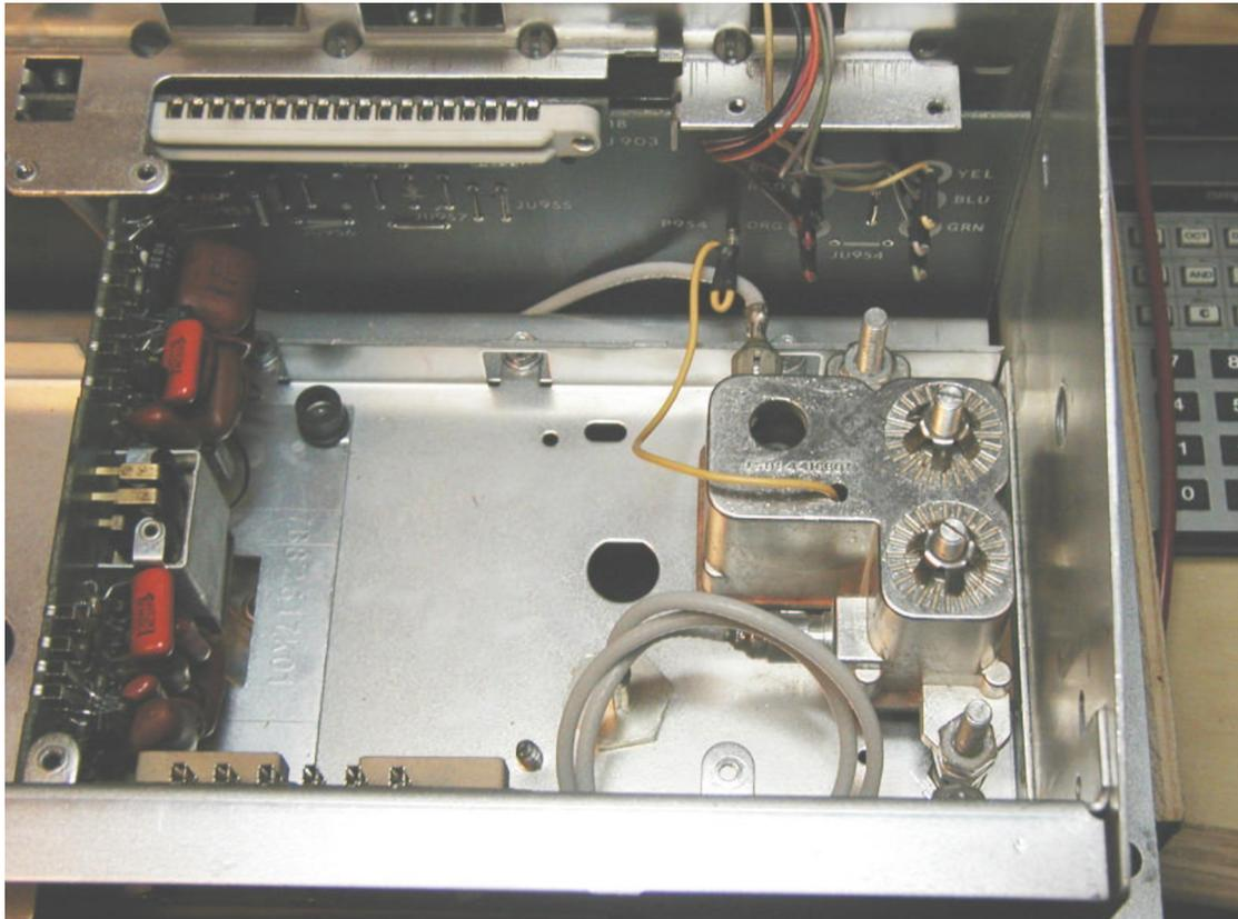
12) Add a 4k7 resistor from J2-10 to ground. This gives a load for the PL detect signal. I found operation with the RLC was intermittent without the pull down. The voltage swing at J2-10 should be 0.3(no PL) to 9.0(PL detected) with the controller plugged in. There is a convenient ground connection down and right of J2-10. Its the heavy trace leaving the J1 power connector.
