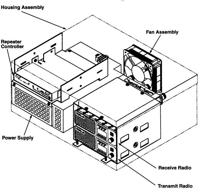
Figure 1-2. GR500 Repeater Station (before mounting)
