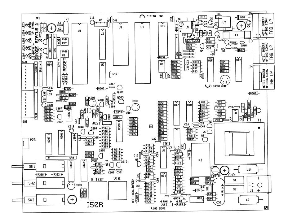
Component Layout Diagram for i50R Basic Interconnect Controller
