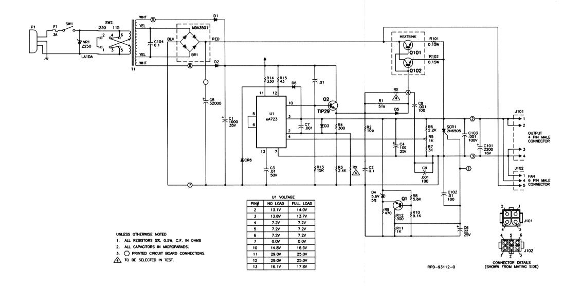
NOTE: THIS IS AN ASTRON SL-14M POWER SUPPLY (IN THIS CASE, THE "M" STANDS FOR MOTOROLA-THERE ARE NO METERS ON THIS UNIT)
