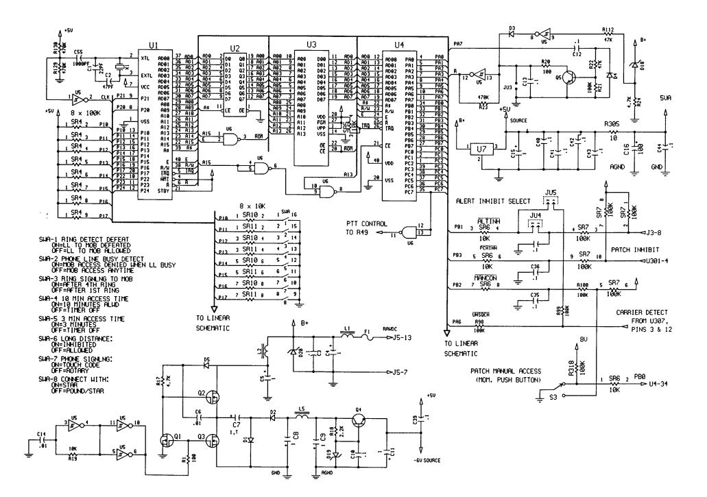
Schematic Diagrams for i50R Basic Interconnect Controller, Power Supply and Digital Section (Sheet 3 of 5)
