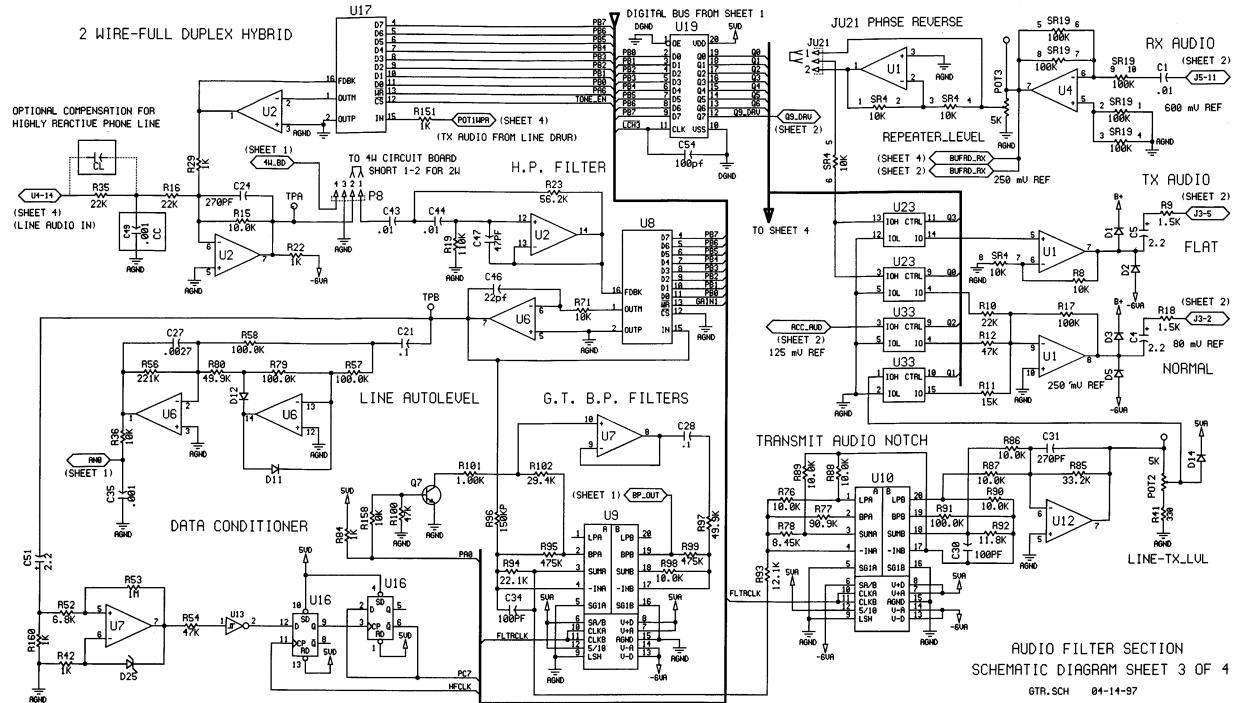
Schematic Diagram for TRA100R Tone Remote Adapter Repeater Controller, Audio Filter Section (Sheet 3 of 4)
