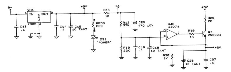
Schematic Diagram for Controller Board for ZR320 Selective Calling Interconnect Controller and ZR330 Remote Telephone Interface Controller
