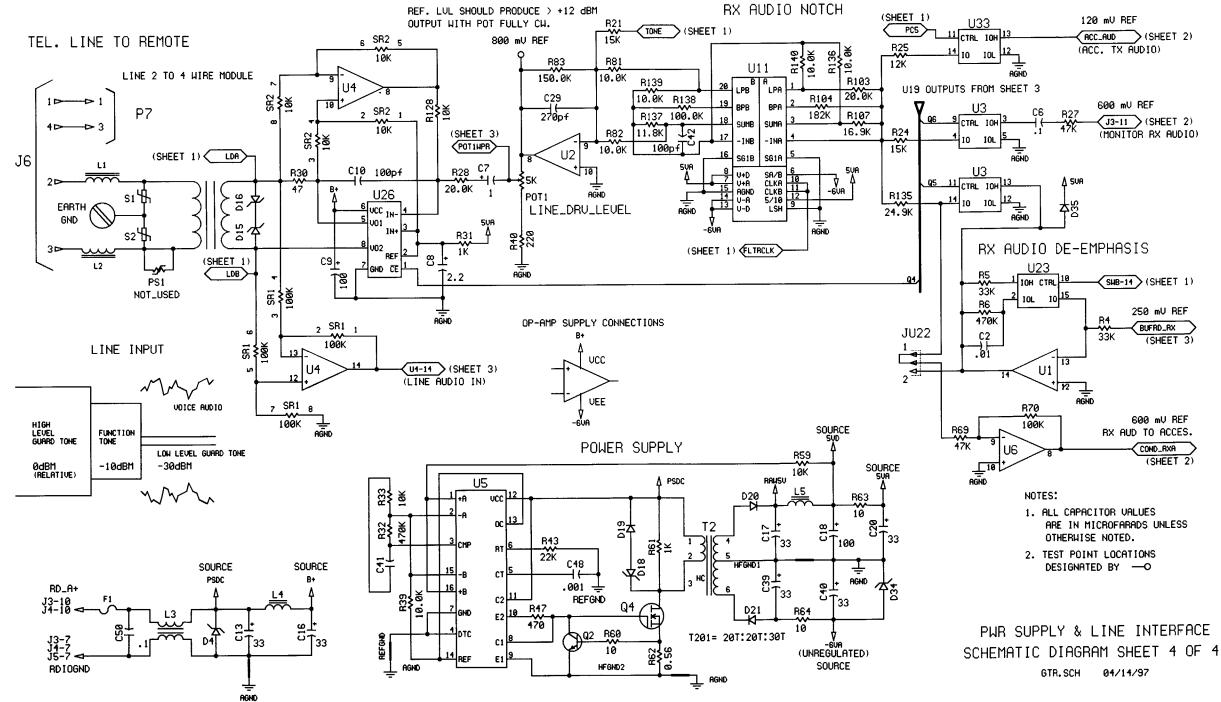
Schematic Diagram forr TRA100R Tone Remote Adapter Repeater Controller, Power Supply & Line Interface Section (Sheet 4 of 4)
