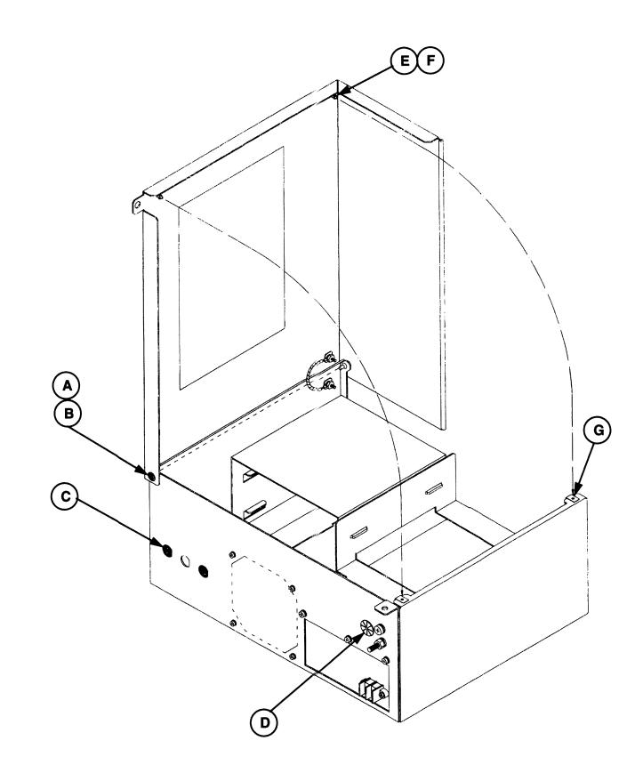
Figure 3-2. GR500 Repeater Station (before wall mounting) Front View Internal Parts
