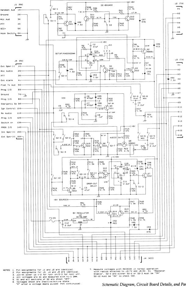
Schematic Diagram, Circuit Board Details, and Parts Lists For Basic Repeater Controller
