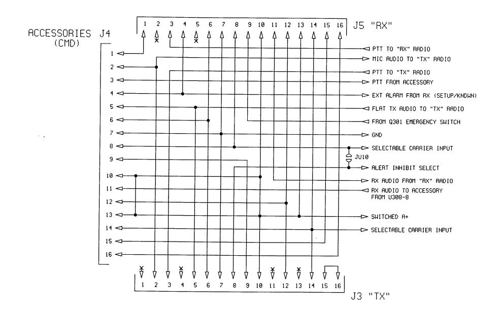
Schematic Diagrams for i50R Basic Interconnect Controller, Interface Schematic Diagram (Sheet 5 of 5)
