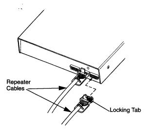
Figure 2-7. Repeater Controller, Rear View
