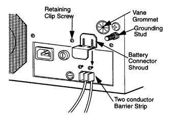
Figure 3-6. Placement of Battery Connector Shroud
