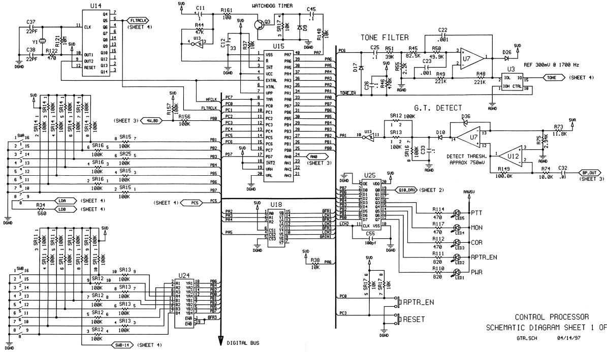
Schematic Diagram and Parts List for TRA100R Tone Remote Adapter Repeater Controller, Controller Processor Section (Sheet 1 of 4)
