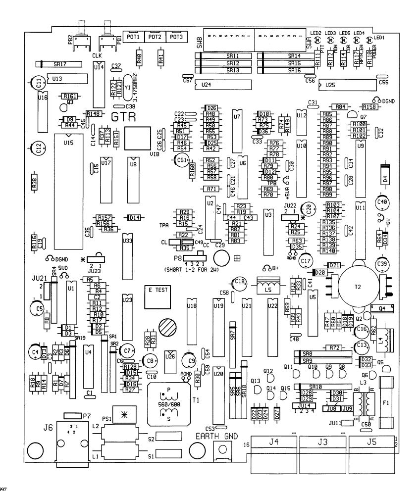
Component Layout Diagram for TRA100R Tone Remote Adapter Repeater Controller
