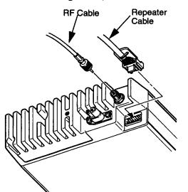
Figure 2-3. GM300 Receive Radio, Rear View
