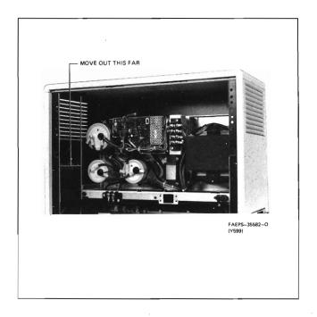
Figure 5. Power Supply Chassis Travel Distance
