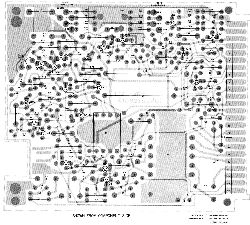
Circuit Board Detail & Parts List Motorola No. 68P81062E41-B (Sheet 1 of 2) 11/1/85-UP
