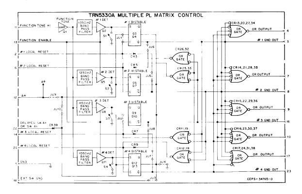
Figure 1. Functional Diagram
