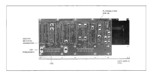
Figure 1. Basic Chassis Exciter Metering Connection Detail
