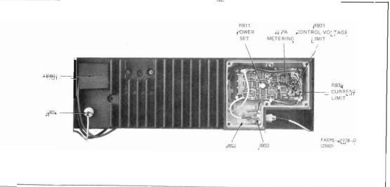
Figure 4. PA Adjustment Location Detail
