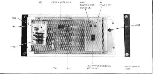
Figure 4. PA Adjustment Location Detail
