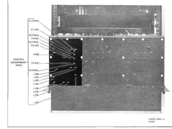
Figure 3. Exciter Adjustment Location Detail
