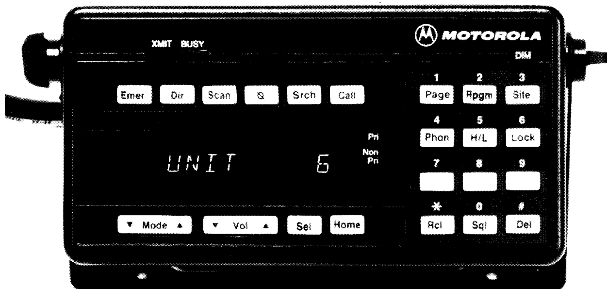
Figure 2. Systems 9000 Control Unit for SYNTOR X 9000E Radios
