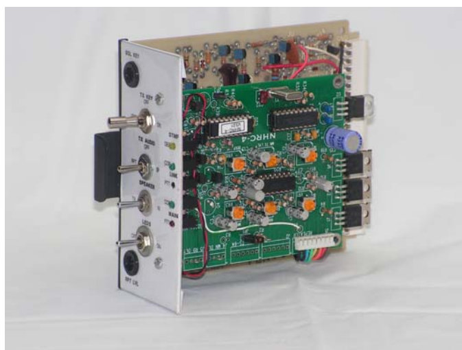
Figure 1 — The YAP 2000 Repeater Controller module is designed to replace the factory Squelch Gate module in an MSR 2000 RF-Control Chassis.
