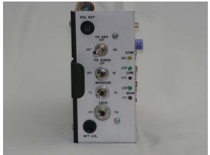
Figure 2 — The new front panel was made from a Line Driver module because it is twice as wide as the Squelch Gate module's front panel and can accommodate both the squelch gate board and the repeater controller board.
