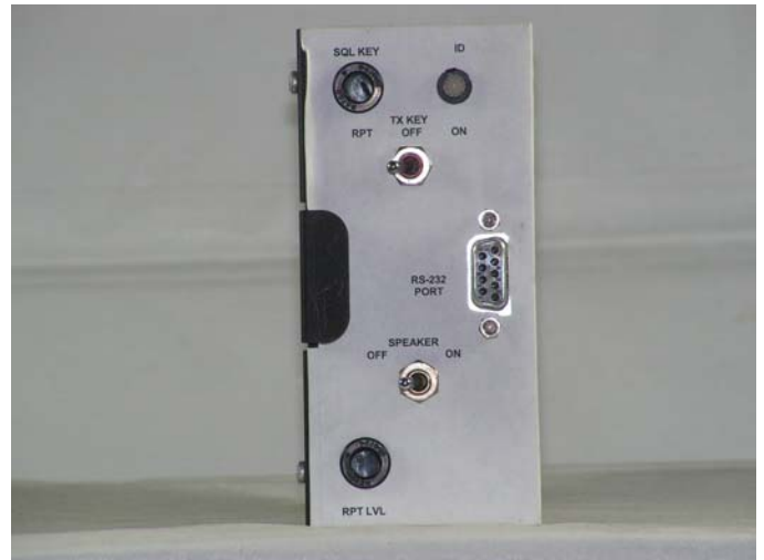
Figure 2 — The new front panel was made from a Line Driver module because it is twice as wide as the Squelch Gate module's front panel and can accommodate both the squelch gate board and the ID-O-Matic II identifier board.
