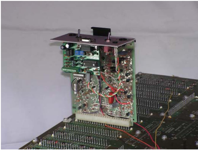
Figure 6 — The YAP 2000 ID module plugged onto the rear of the backplane in the Squelch Gate module position. If you do this, there are two caveats you need to be aware of: First, you should only insert a module onto its own backplane connector; otherwise, it may not function properly and it may be damaged. Second, you have to pay attention that you don't insert the module up-side-down, i.e., pin 1 to pin 24.
