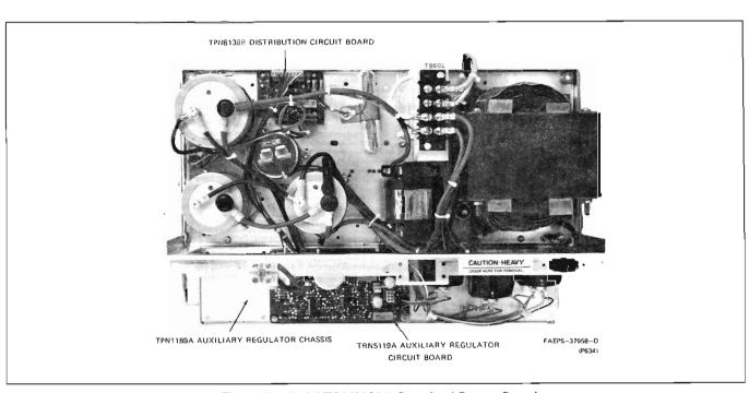
Figure 1. Model TPN1191A Standard Power Supply
