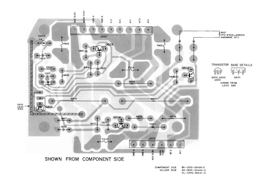
TRN5336A Standard Power Supply, and TRN6138B Distribution Board Schematic Diagram, Circuit Board Details, and Parts Lists Motorola No. PEPS-34737-C (Sheet 1 of 2) 1/14/83 · V & G
