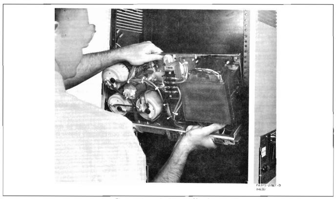
Figure 4. Properly Gripped Chassis
