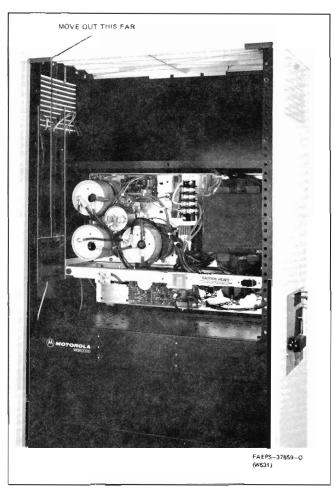
Figure 3. Power Supply Chassis Travel Distance
