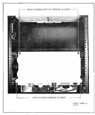
Figure 2. Power Supply Mounting Hardware
