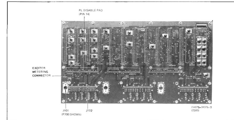
Figure 2. Fully Optional Chassis Exciter Metering Connection Detail
