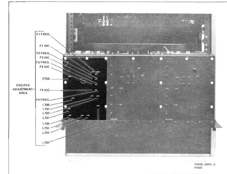
Figure 3. Exciter Adjustment Location Detail
