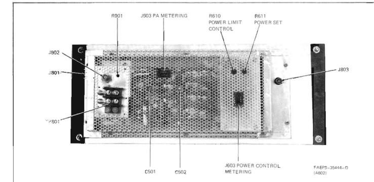
Figure 4. PA Adjustment Location Detail
