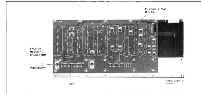
Figure 1. Basic Chassis Exciter Metering Connection Detail
