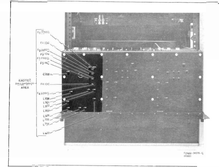
Figure 3. Exciter Adjustment Location Detail
