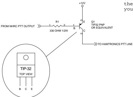
All NHRC products have active low PTT closure to ground. This simple circuit will key an active high transmitter such as a Hamtronics product.
