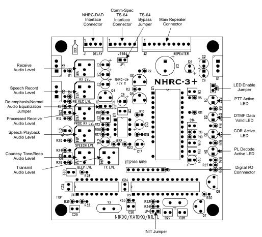
The following diagram is a detailed top view of the Revision "C" printed wiring board for the NHRC-3+ Repeater Controller.
