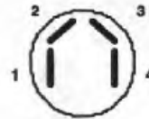
SELECT SWITCH (SW) (view onto rear pins)
