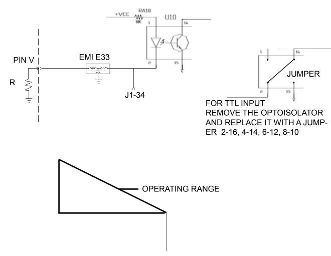
The minimum resistance to ground to produce an active COR is 7.5k or at least 0.5 mA is required.
