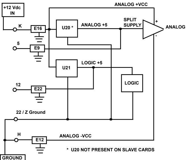
**Pin 5 = Analog split supply out to slave cards** Pin 12 = +5v Logic out, not tied to slave
