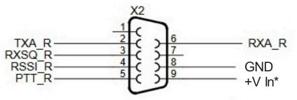
\*+V In pin only applicable on V3 boards, Otherwise, cut wire for pin 9.
