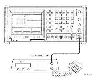
Connect the COM-120B T/R connector to the Unit Under Test (UUT) TRANSMIT OUT via a coaxial cable.
