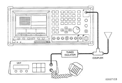
This procedure configures the RF Receive Operation Screen to measure Isolation and Insertion Loss.
