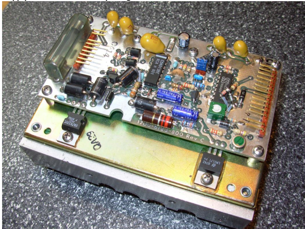
Inverter Supply with attached battery charger board removed from IFR 1200S
