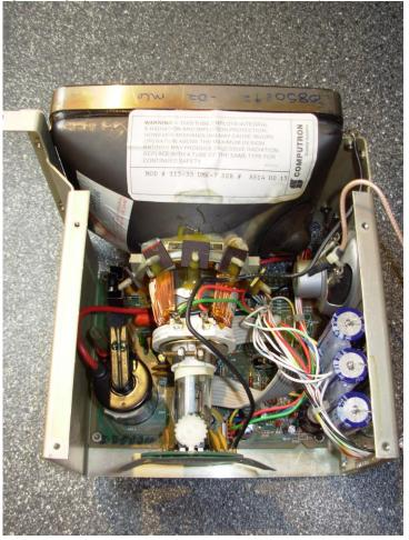
As pictured above the Computron CRT Display Module is one chassis with one coax cable (speaker audio cable) and one wire harness connector connecting it to the main body of the IFR A-7550. The CRT module can be removed after removing the front panel of your A-7550, unplugging the two keyboard ribbon connectors, Speaker SMB connector, and front panel SMA connectors, and removing 5 screws that hold the CRT module (as pictured above) in the body of the A-7550.
