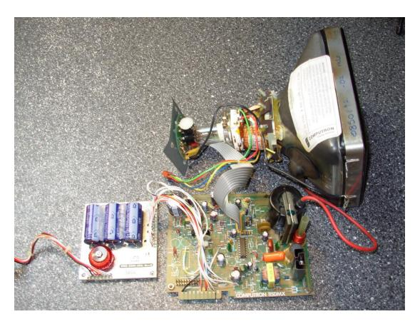
Once the A-7550 CRT Module is removed from the main chassis of the A-7550 the entire assembly can be disassembled further. There are 4 screws holding the CRT to the frame, 4 screws holding the Computron 115DMX board to the chassis, and 4 screws holding the IFR CRT Filter PC board to the chassis. Once all 12 screws are removed you can slide everything out the front of the frame and lay the boards out for capacitor removal.
