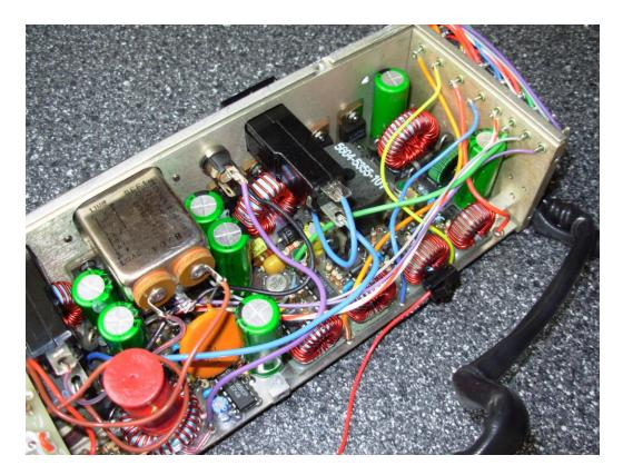
IFR A-7550 Power Supply Capacitor List All capacitors in the power supply were upgraded to 105 deg C rating when available.
