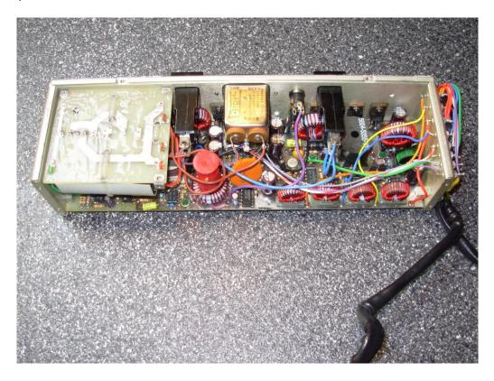
External power supply axial lead electrolytic capacitors from top to bottom (Renewal Optional) C9- 1000uF, 6.3V, 20%, Axial Lead, 85deg Replacement Manufacturer: Nichicon Replacement Part Number: TVX0J102MCD Quantity on Board: 1
