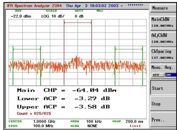
The measurement results are displayed on the lower part of the screen. Correcting the measurement will start with calculating the average value of adjacent channel power differences.
