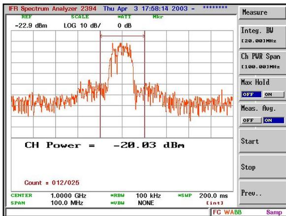
On top of that, each sample must represent a real sample: when entering this measurement mode, the spectrum analyzer automatically switches to the "Sample" detection mode. The power measurement is processed using real samples taken at the display points (different from the normal spectrum analyzer mode where "Peak Pos" is normally used).
