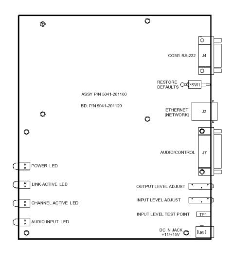
Figure 2-3 NXU-2A Internal View
