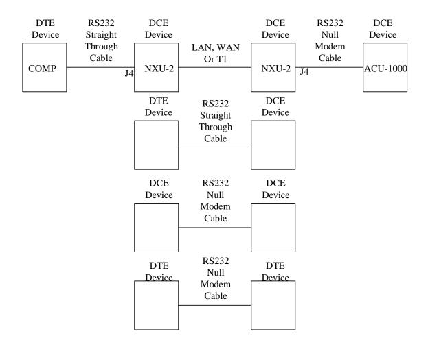
Figure 2-4 DTE Versus DCE Serial Cables
