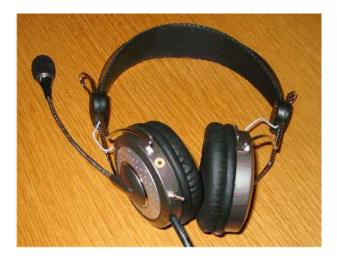
The original headphone cable has been removed and replaced with a length of pre-terminated CAT5 patch cord. I modified this by splicing the cable at about 50mm away from the end with the RJ45 connector.
