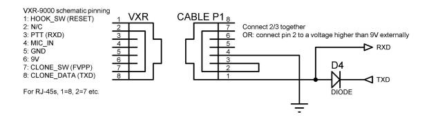
Final VXR-9000 programming cable design for standard TTL UART connection (e.g. USB serial dongle).
