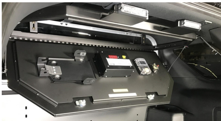
Figure G-4 Example of SUV Fold Away Mounting System (Photo Courtesy of Lund Industries)
