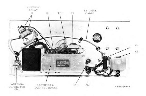
Power Amplifier (Rear View) Alignment and Parts Location Detail
