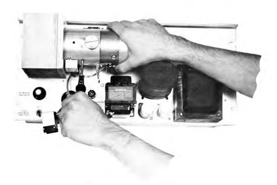
Power Amplifier Tube Removal Detail A
