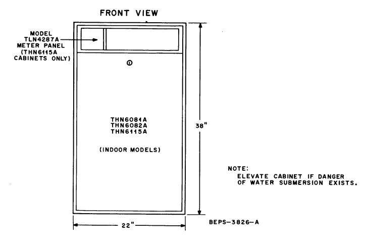
Models THN6082A and THN6115A "Compa-Station" Base Radio Cabinet Dimensional Detail Motorola No. BEPS-3826-A 8/6/74-NPC
