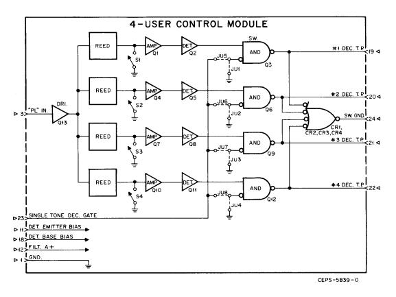
4-User Control Module Functional Block Diagram
