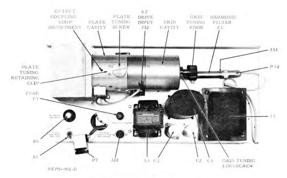
Power Amplifier (Front View) Alignment and Parts Location Detail
