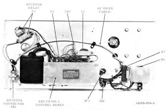
Power Amplifier (Rear View) Alignment and Parts Location Detail
