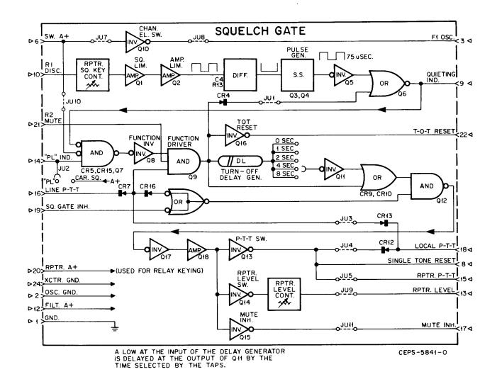
during a received rf signal or during the timed delay period. However, this switch is not enabled in the local or wire line control modes and the receiver will be muted.
