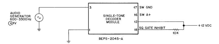
Test Set Up Diagram
