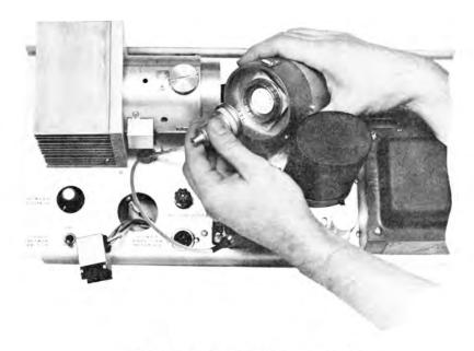
Power Amplifier Tube Removal Detail B
