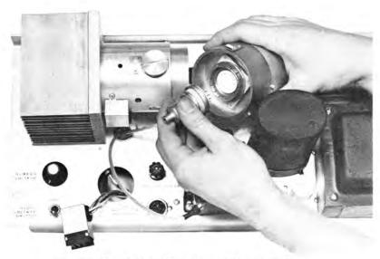
Power Amplifier Tube Removal Detail B
