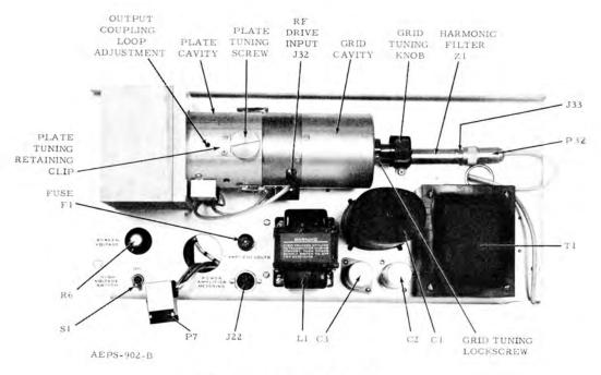
Power Amplifier (Front View) Alignment and Parts Location Detail
