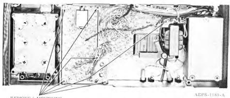
REMOVE 6 MOUNTING SCREWS AND FOLD OUT BOTH BOARDS TOGETHER.
