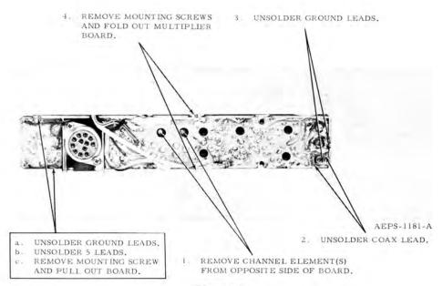
Figure 8. Access to Multiplier and Regulator Boards
