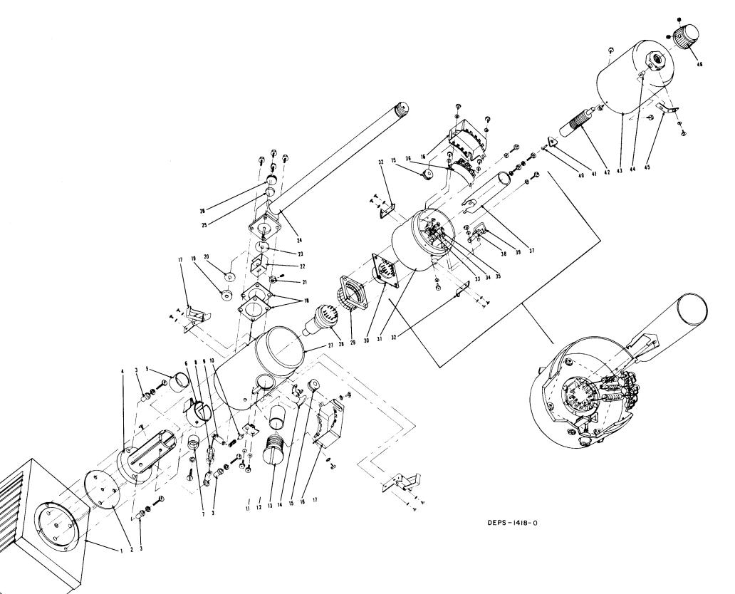
Power Amplifier Cavity Mechanical Parts Detail Motorola No. PEPS-1710-B 6/5/74-NPC
