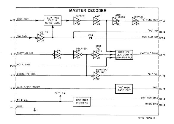
Master Decoder Module Functional Block Diagram
