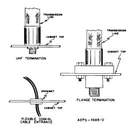
Figure 2. Indoor Cabinet Antenna Cable Installation
