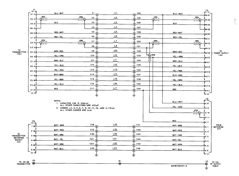
TLN8888B Transmitter Shield Schematic Diagram Motorola No. 63C81102E57-A 8/6/74-NPC
