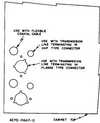
Figure 1. Cabinet Knockout Detail
