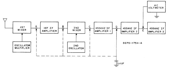
Figure 3. "Noise Gain" Measurement Test Set-Up
