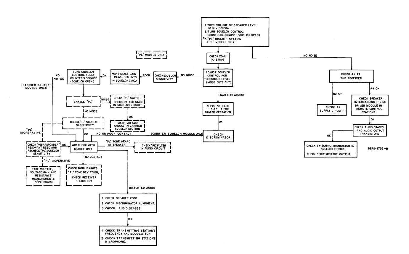
Individual stages can be checked by injecting an audio signal and measuring signal voltages at each stage. Set the receiver VOLUME control to maximum and the SQUELCH control fully counterclockwise (unsquelched). On "Private-Line" tone-coded squelch models, also "PL" disable. Inject a 1000-Hz tone at 0.4 volt rms into the audio board (input from discriminator). The Motorola SLN6221A Transistorized Tone Generator is ideal for generating this tone.
