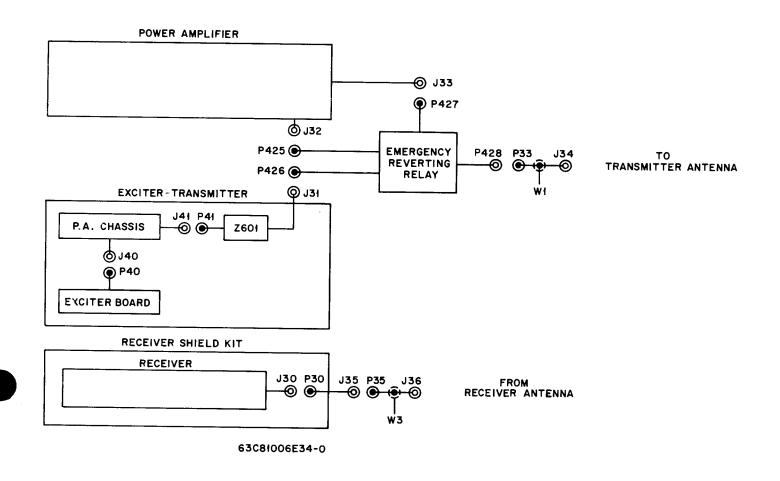
RF Intercabling Diagram with Emergency Power Reverting Motorola No. 63C81006E34-O 8/6/74-NPC
