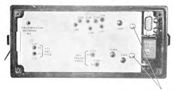
TO GAIN ACCESS TO PLATED SIDE OF CHASSIS, REMOVE SCREWS
