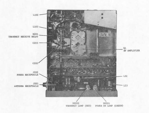
Carrier Squelch Models Parts Location Detail Bottom View
