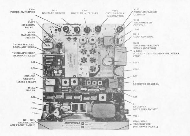
$\begin{array}{c} {\bf Dual\ Squelch\ Models\ Parts\ Location\ Detail} \\ {\bf Top\ View} \end{array}$
