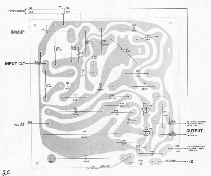
Dual Squelch Receiver, Model TLN6727A-1 Tone & Noise Amplifier Printed Board and Wiring Diagram Motorola No. EPD-9346-D 12/15/64-RCS CEPD-9344-A DEPD-9345-D p/o 63E81018A97
