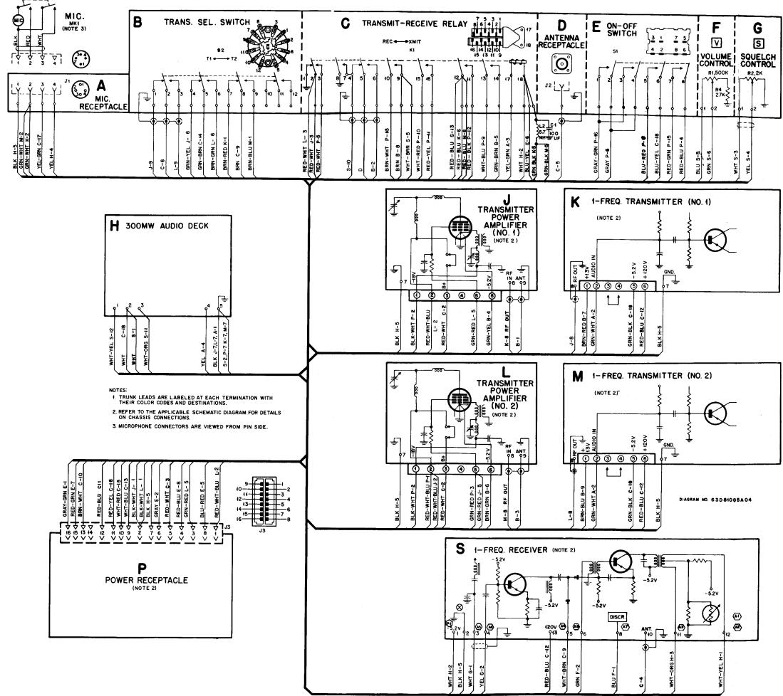
"P" Series "Handie-Talkie" Radiophones W/Two 1-Freq. Transmitters Intercabling Diagram Motorola No. 63D81005A04-E
