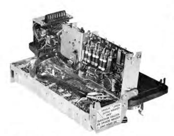
Figure 4. Transmitter in Service Position
