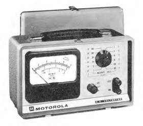
Transistorized AC Voltmeter
