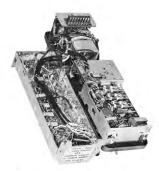
Figure 3. Receiver in Service Position
