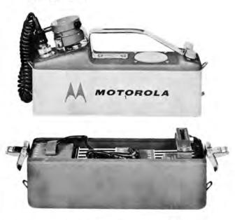
Figure 1. Battery Section Removed
