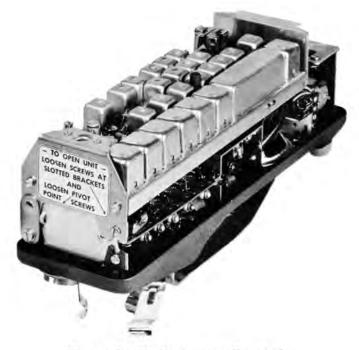
Figure 2. Radio Section Exposed
