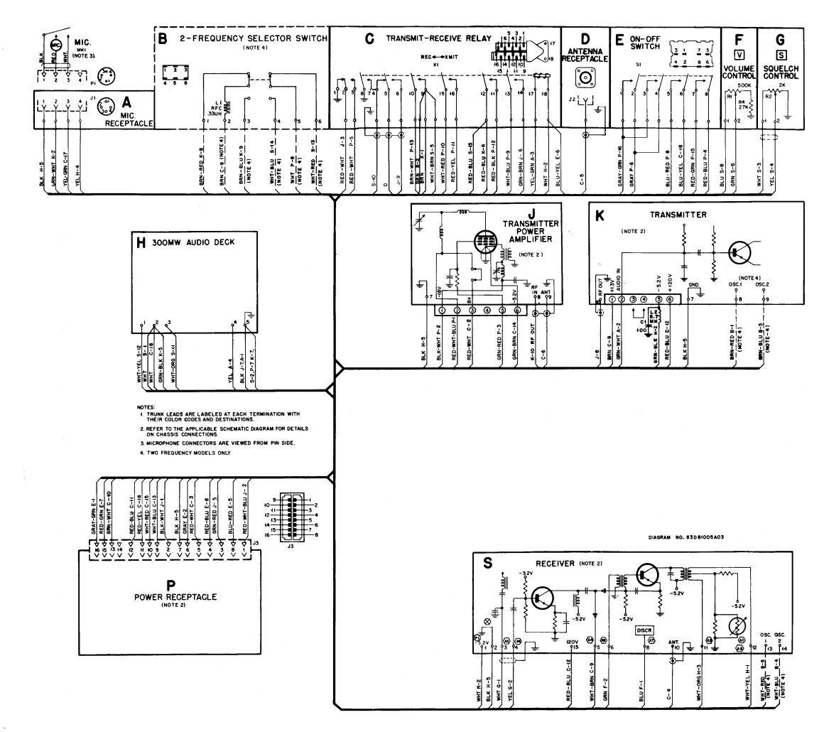
"'P" Series "Handie-Talkie" Radiophones W/l or 2-Freq. Receiver and One l or 2-Freq. Transmitter Intercabling Diagram Motorola No. 63D81005A03-D PARTS LIST for Intercabling Diagram 63D81005A03-D
