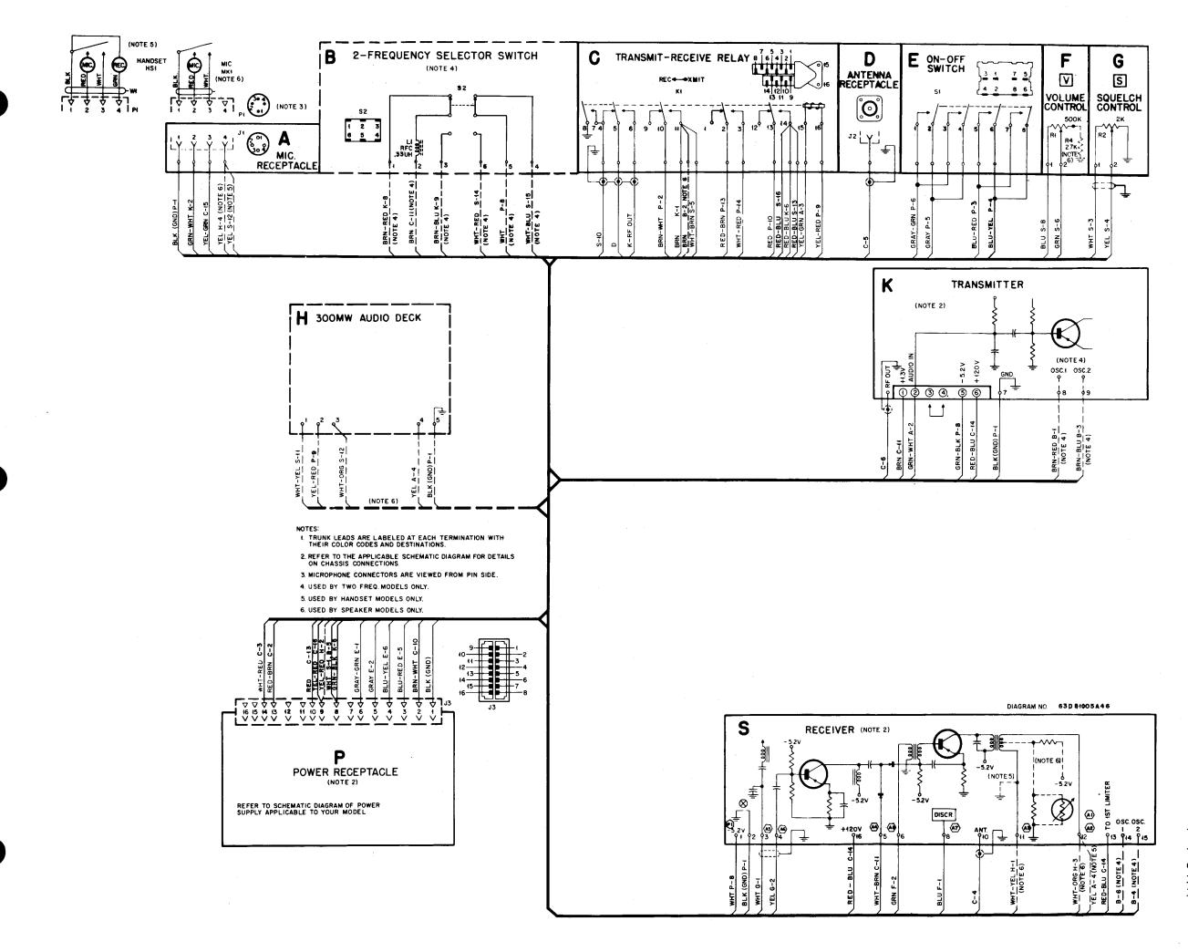
"H" Series "Handie-Talkie" Radiophone W/l or 2-Freq. Receiver and One l or 2-Freq. Transmitter Intercabling Diagram Motorola No. 63D81005A46-D
