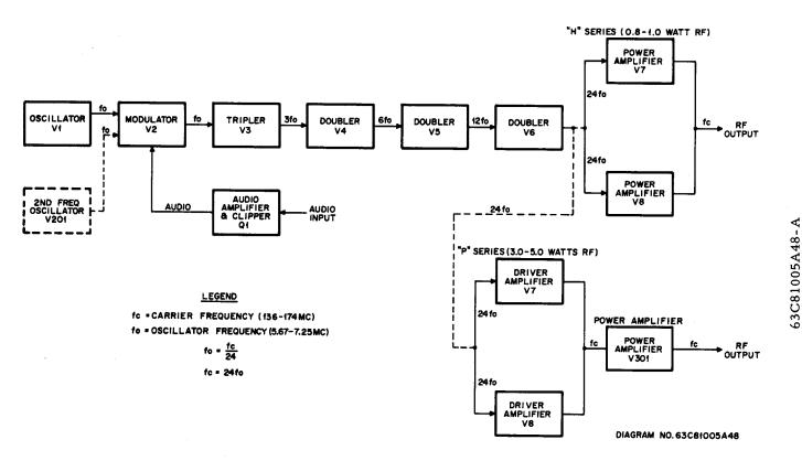
Transmitter Block Diagram
