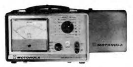
Transistorized AC Voltmeter
