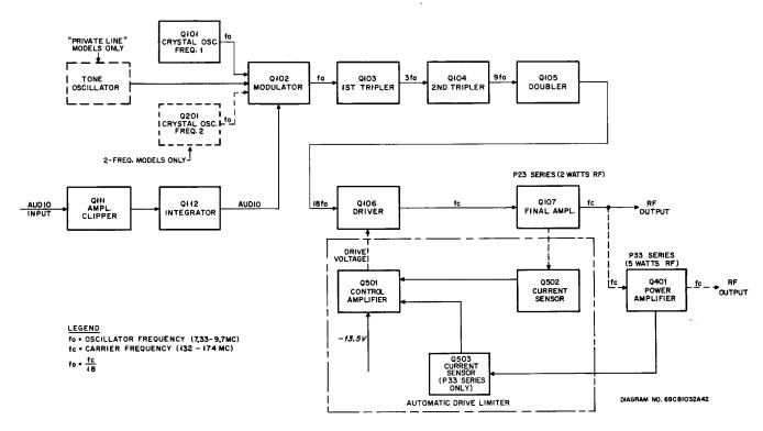
Transmitter Block Diagram
