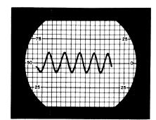
(2) With this input signal level, adjust the IDC control on the transmitter to provide a 10-square peak-to-peak recovered signal on the oscilloscope. This is equivalent to ±5 kc deviation as shown in figure 2.
