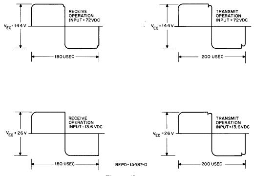
Figure 41. Power Supply Converter Waveforms
