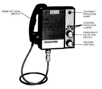
Figure 17. Non-Reverting Standard AAR Control Head
