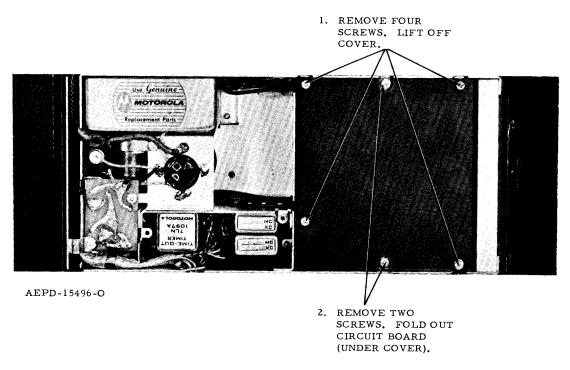
Figure 44. Access to Components on Switching Circuit Board
