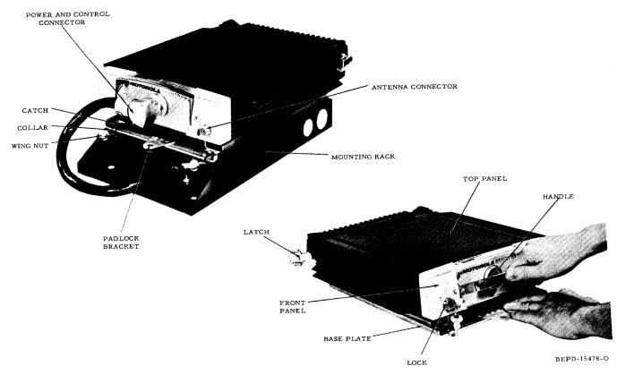
Figure 24. Identification of Parts for Standard AAR Housing Removal and Replacement
