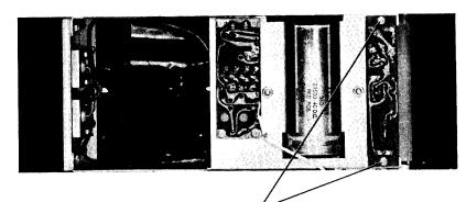
REMOVE TWO(2) MOUNTING SCREWS AND FOLD OUT PRINTED CIRCUIT BOARD.
