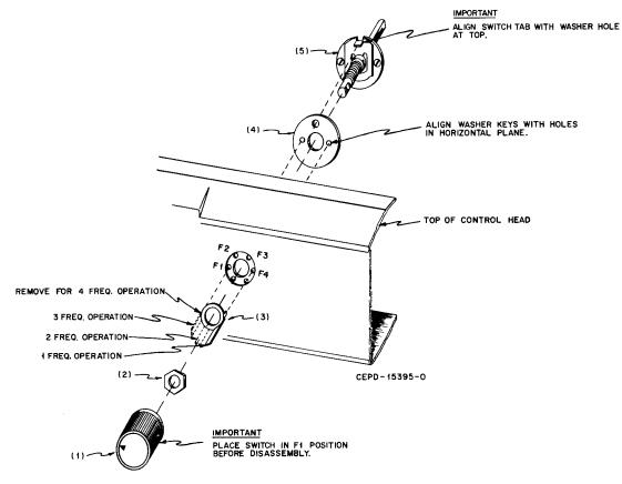
Figure 16. Universal Control Head Frequency Selector Switch Stop Detail
