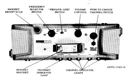
Figure 18. Channel Reverting Universal Control Head With "Private-Line" Tone-Coded Squelch
