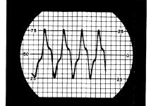
Figure 2. 5 KC Peak Deviation as seen on the Oscilloscope (NOTE: Waveform is clipped fully)
