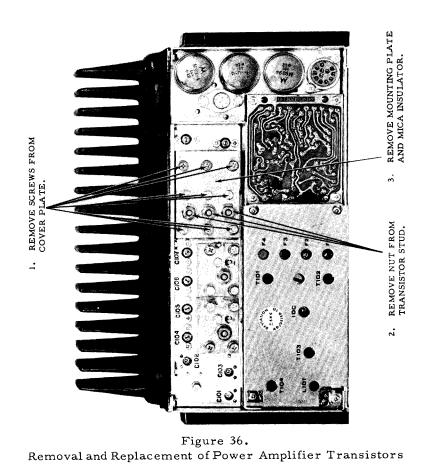
4. UNSOLDER PA TRANSISTOR LEADS AND REMOVE TRANSISTOR.
