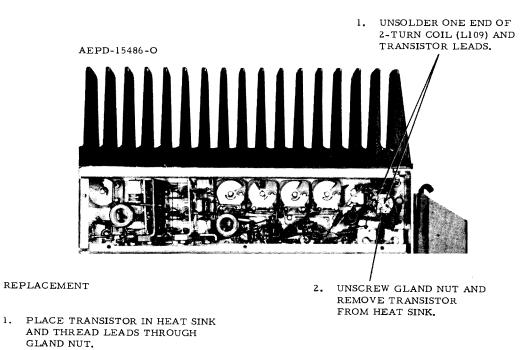
SCREW ON GLAND NUT AND SOLDER TRANSISTOR LEADS AND 2-TURN COIL (L109) IN PLACE.
