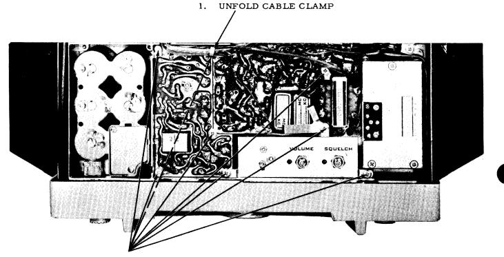
2. REMOVE MOUNTING SCREWS AND CAREFULLY FOLD OUT BOTH BOARDS TOGETHER. ALSO FOLD OUT VOLUME AND SQUELCH DECK. USED CARE WHEN FOLDING OUT BOARDS TO ASSURE INTERCONNECT-ING LEADS ARE NOT BROKEN.
