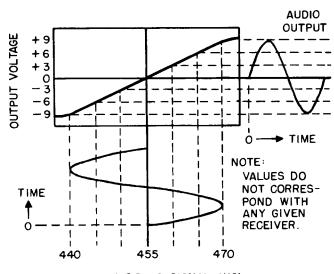
FREQUENCY OF I-F SIGNAL (KC) Figure 21. Typical Discriminator Response
