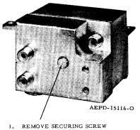
REMOVE SECURING SCREW AND PULL ANTENNA SWITCH-ING NETWORK FROM HAR-MONIC FILTER.
