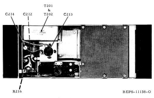
Figure 45. Power Supply Miscellaneous Parts Location
