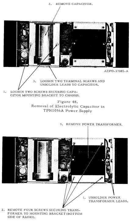
Figure 49. Removal of Power Transformer in TPN1056A Power Supply
