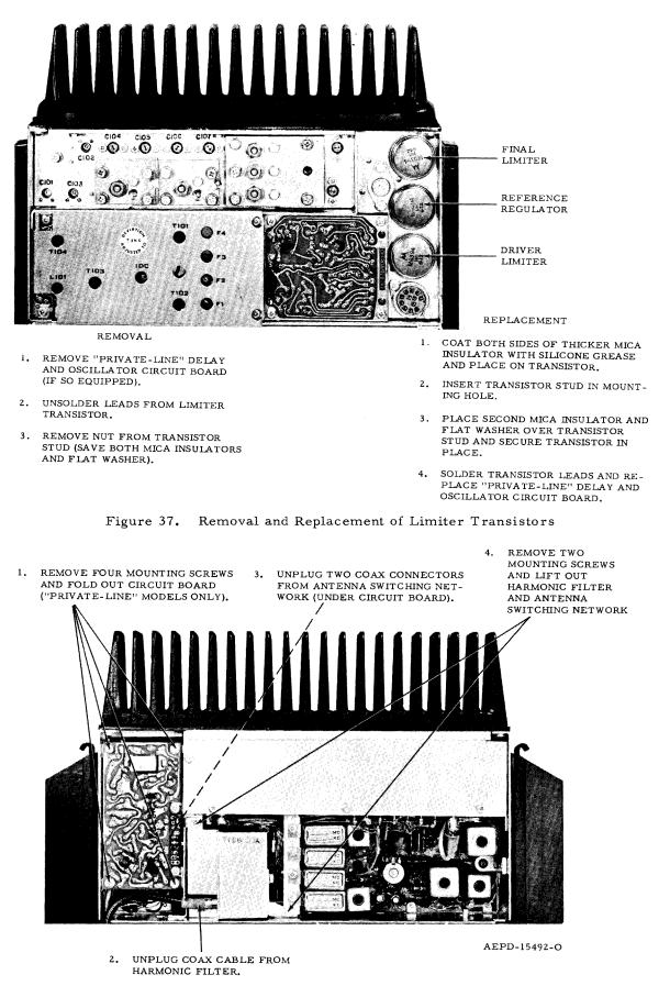
Figure 38. Removal of Harmonic Filter and Antenna Switching Network
