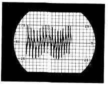
Figure 3. 5 KC Peak Deviation for Combined "PL" Tone and 1000 cps Modulation (NOTE: "PL" Tone Superimposed on 1000 cps tone)
