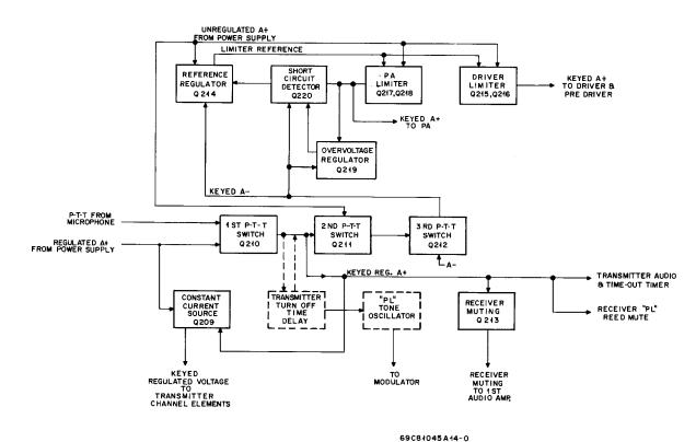
Figure 23. Transmitter Switching Circuits Block Diagram
