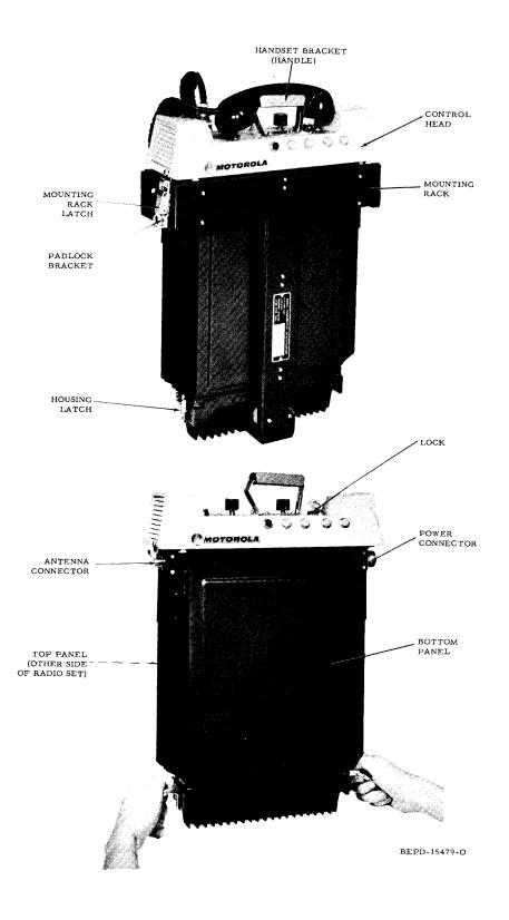
Figure 25. Identification of Parts for Universal Housing Removal and Replacement
