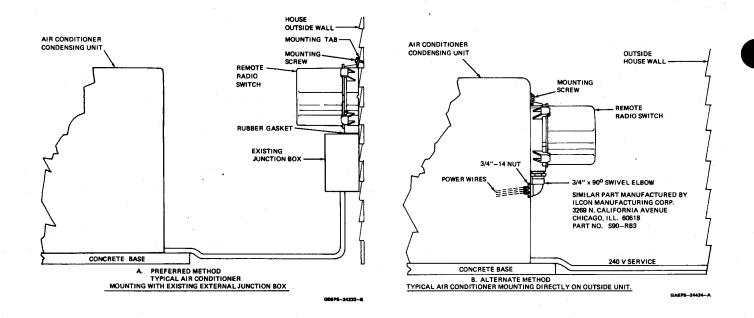
Figure 3. Typical Air Conditioner Installations
