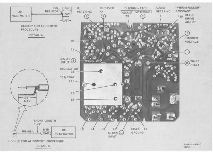
Figure 11. Alignment and Test Point Locations
