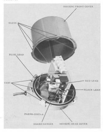
Figure 9. Housing and Board Removal
