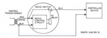
Figure 8. 24 V ac Thermostat Control Circuit Installation Wiring
