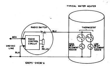
Figure 6. Standard 240 V ac Installation Wiring
