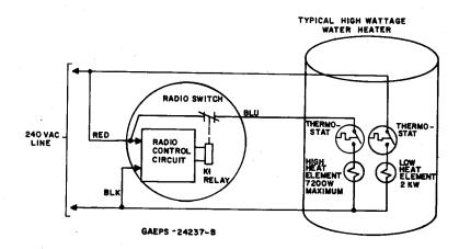
Figurè 7. Typical 240 V ac High Wattage Heater Single Element Control, Installation Wiring
