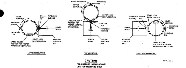
Figure 5. Remote Radio Switch to Junction Box Mounting Details
