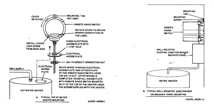
Figure 4. Typical Hot Water Heater Installations
