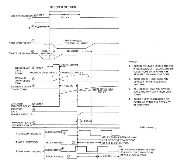
Remote Radio Switch Mechanical Parts Details and Timing Diagram Motorola No. PEPS-28283-O 2/22/79-
