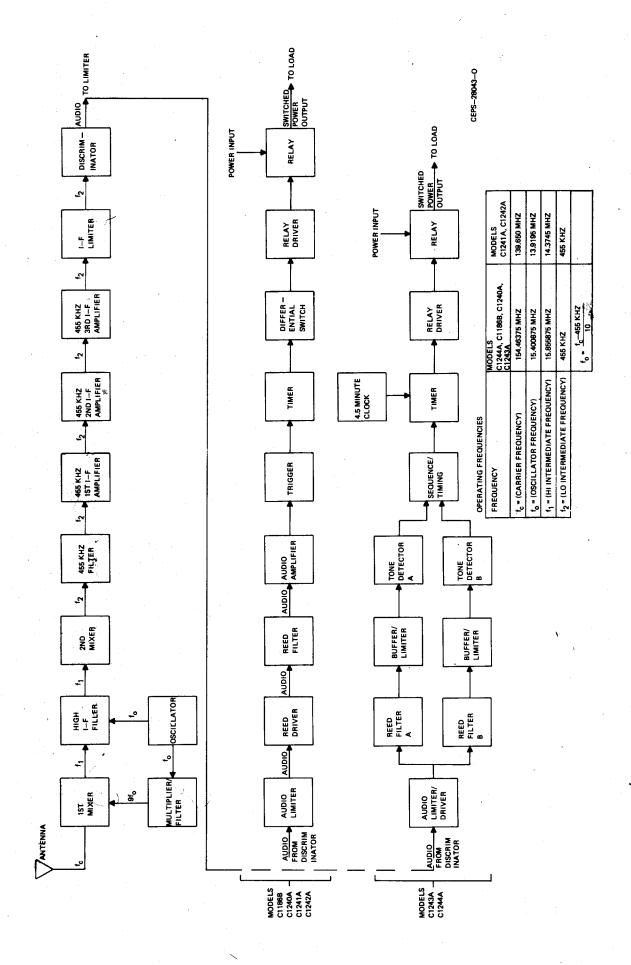
Figure 1. Block Diagram of Radio Switch
