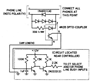
Least Cost Routing Through Your PBX. Chris Boon, WB5ITT, points out a nice feature of Version 3 with your RC-850 controller if you're connected to a PBX. Certain calls can be automatically routed to different tie lines, using the multiple "logical phone lines" of the controller, and its telephone exchange tables to make the routing decision.
