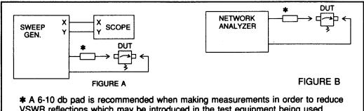
VSWR reflections which may be introduced in the test equipment being used. (Optional-Depending upon equipment being used).
