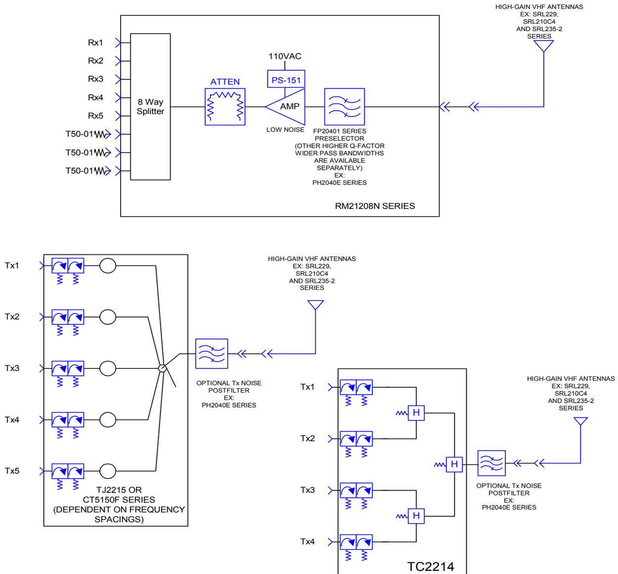
**Note:** Sinclair can customize the antenna system based on the site requirements of the customer. Some customizations include: single antenna systems using a duplexer or multiple antennas, varying number of channels, high-power, simplex and half-duplex radio combining, cabinets, C-series through-line combining. Contact your Sinclair representative or Systems Engineer for details.
