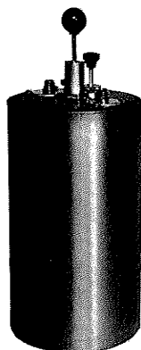
TYPICAL RESONANT CAVITY SHOWING SEPARATE COARSE AND FINE TUNING CONTROLS
