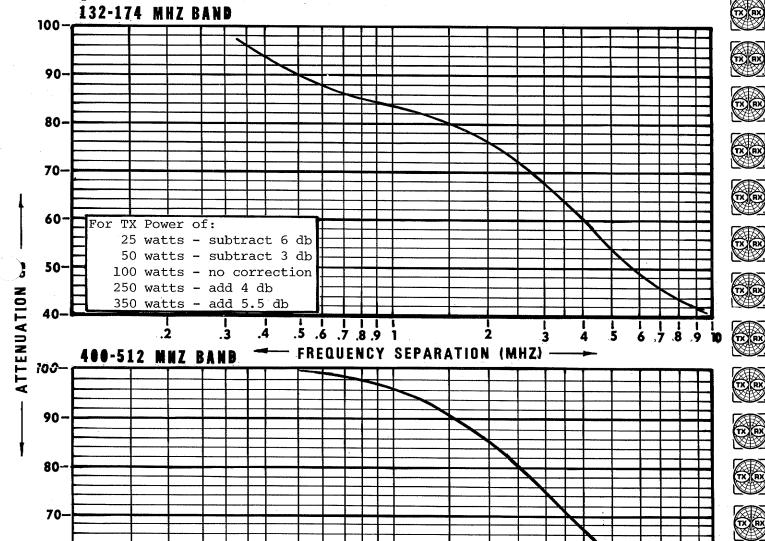
Note: These are only "typical" curves. When accuracy is required, consult the radio manufacturer. **Z(H)402L8**
