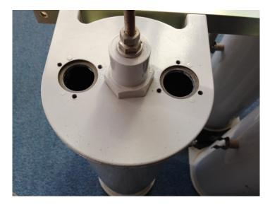
Completed installation of loops, JAG Engineering recommended that the cable length be 12.726" for RG-142 or 12" for RG-213 including the connectors. I went with the RG-142 and it appears to be a ¼ wave including the loops and they were spot on as the tuning did not change when the two cavities were interconnected.
