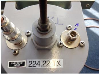
The receive side was adjusted to 1.5 db insertion loss per cavity so I could get steeper skirts on the band pass about -70 dBm at 5 Mhz. The higher loss was not an issue since I was also installing an Angle Linear preamp to make up for the insertion loss after the filters and still have some gain.
