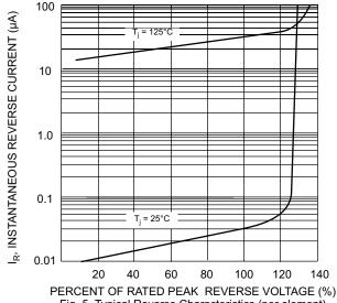
Fig. 5 Typical Reverse Characteristics (per element)
