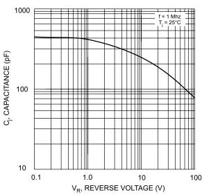
Fig. 4 Typical Junction Capacitance (per element)
