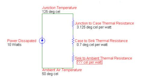
Fig A - Schematic Diagram for Power Dissipation of TIP32C pass device.
