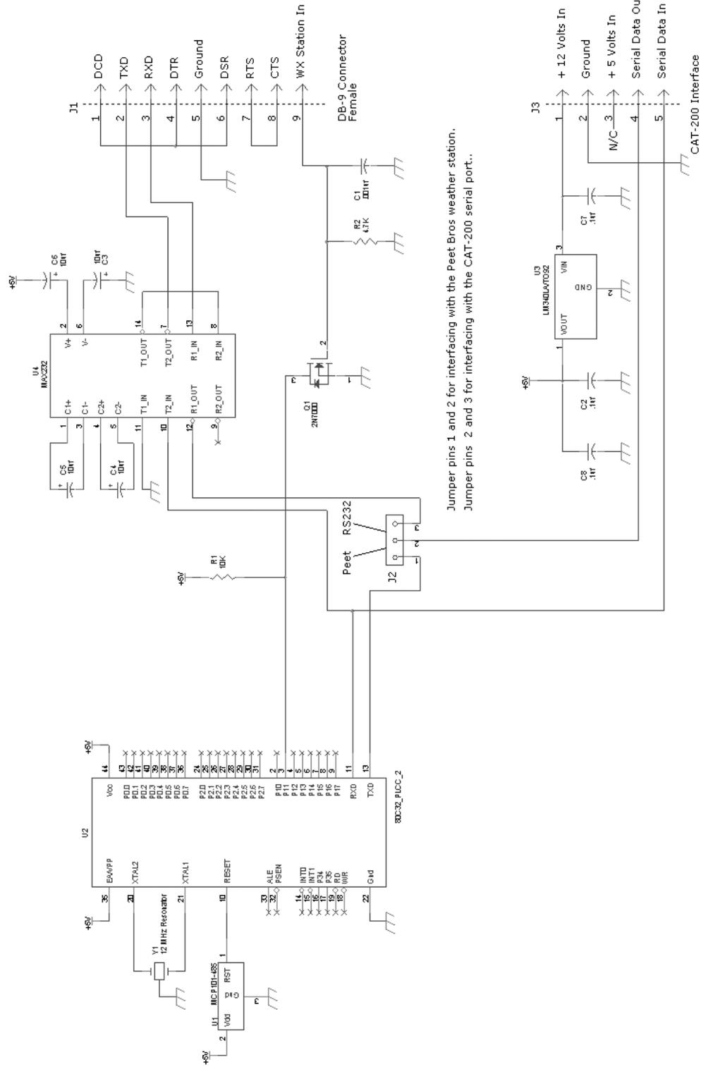
Jumper pins 1 and 2 for interfacing with the Peet Bros weather station.
