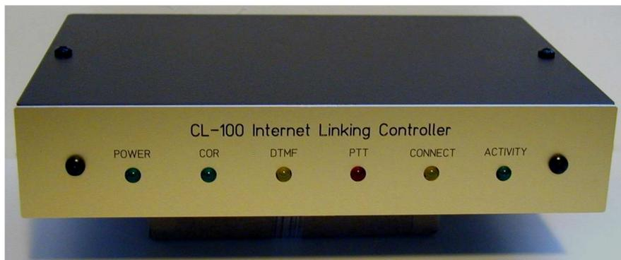
During a firmware upgrade when all four dipswitches are turned on and power is applied the COR, DTMF, PTT, CONNECT and ACTIVITY LEDs will strobe three times to indicate the CL100A has entered into the boot loader mode.
