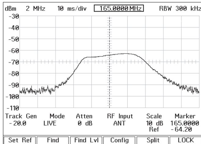
Enter the correct RF frequency and ensure the receiver is turned on. The filter waveform will appear on the scope display. To tune the Front End filter, remove the dust caps on the variable capacitors and, starting from the capacitor closest to the front panel and moving back, tune the filter to its new frequency.
