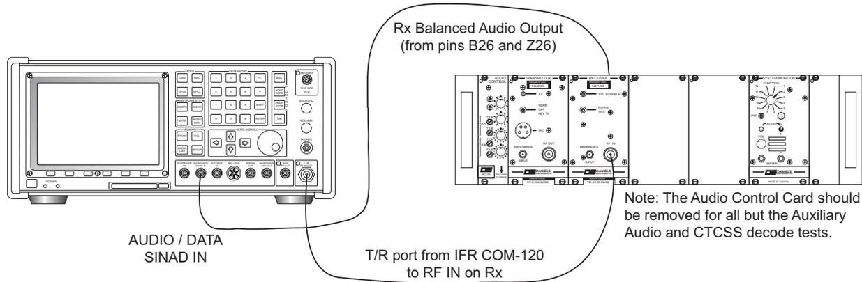
Select the GEN MODE button and set up the IFR COM-120 as follows:
