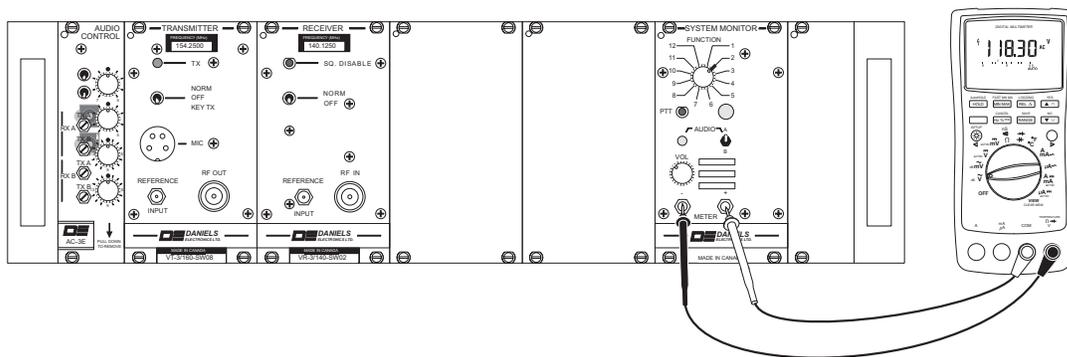
The FUNCTION rotary switch on the front panel of the System Monitor will allow you to test various points in the radio system. Following is a list of System Monitor rotary switch positions, the functions they measure and the parameters measured (please note that switch positions 4, 5, 11 and 12 require a carrier injected into the receiver and position 8 requires an audio tone as well):
