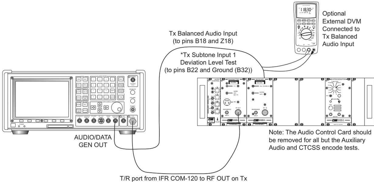
Select the REC MODE button and set up the IFR COM-120 as follows:
