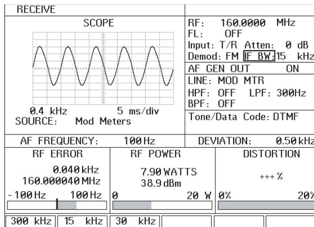
Adjust the Transmitter CTCSS deviation for +/-0.50 KHz wide / +/-0.35 KHz narrow (the adjustment pot is located directly on the CTCSS module in the audio control card). The CTCSS encode tone is the AF Frequency.
