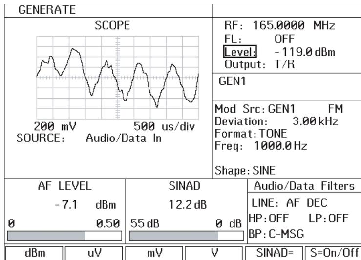
If the Distortion or SINAD measurements are not within Daniels published specifications, the Front End may need re-alignment. Refer to the Receiver Front End Alignment and Tuning section.
