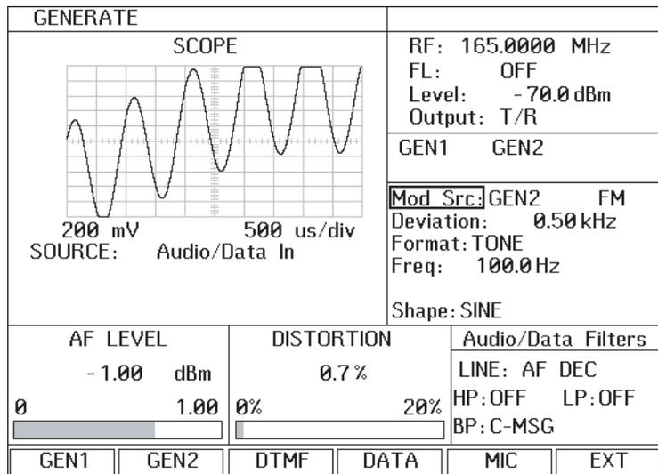
The receiver will now un-mute and the 1 KHz tone (and possibly the CTCSS tone) will be audible on the System Monitor speaker. If the receiver does not un-mute, check that the correct CTCSS tone frequency is entered in the IFR COM-120.
