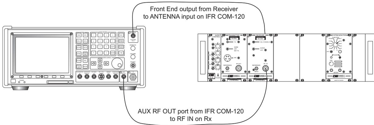
The internal cable in the receiver from the output of the front end terminates in an SMB connector. The SMB plugs directly into the Receiver 21.4 MHz IF / Audio Main Board. Disconnect the SMB cable from the Main Board connector and use the SMB-BNC adapter to connect this point to the ANT input on the IFR COM-120.
