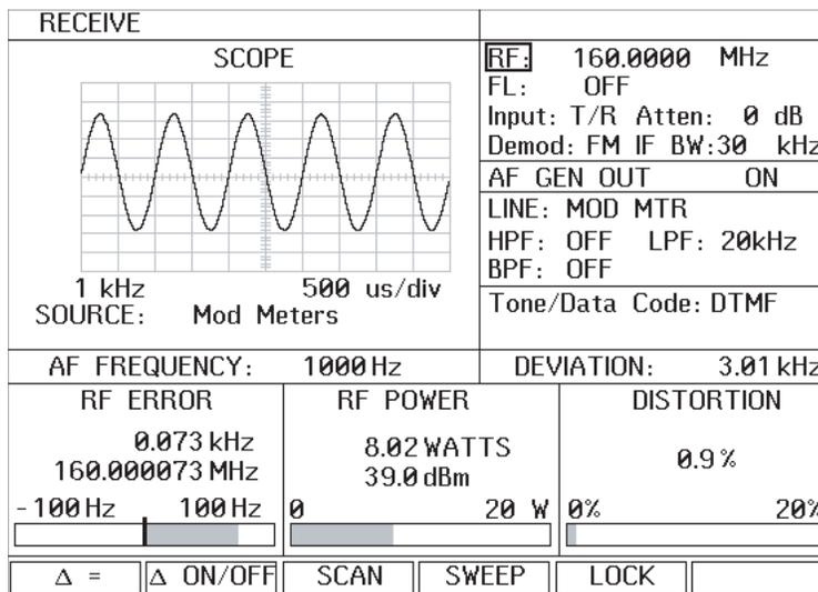
Enter the correct RF frequency, and ensure that the transmitter is set to KEY TX and the Audio Control Card is NOT plugged into the subrack. Set the receive audio filters and AF Generator frequency and level as shown on the next page.
