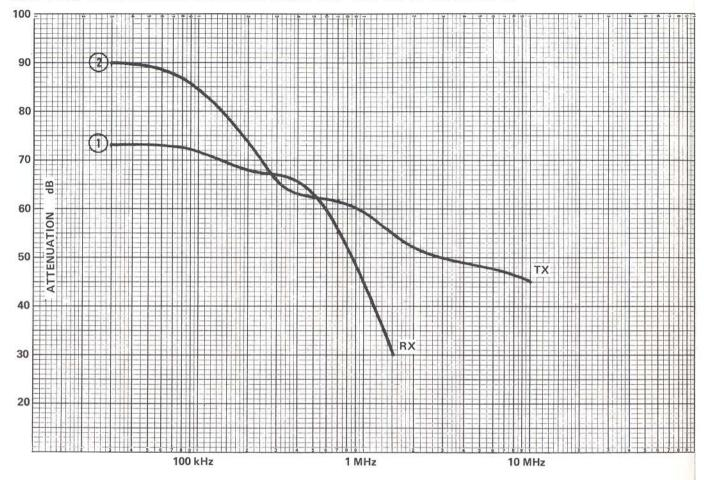
THESE CURVES SHOW THE ATTENUATION REQUIRED TO PREVENT GREATER THAN 1 dB REDUCTION IN A 12 dB SINAD RATIO, DUE TO:
