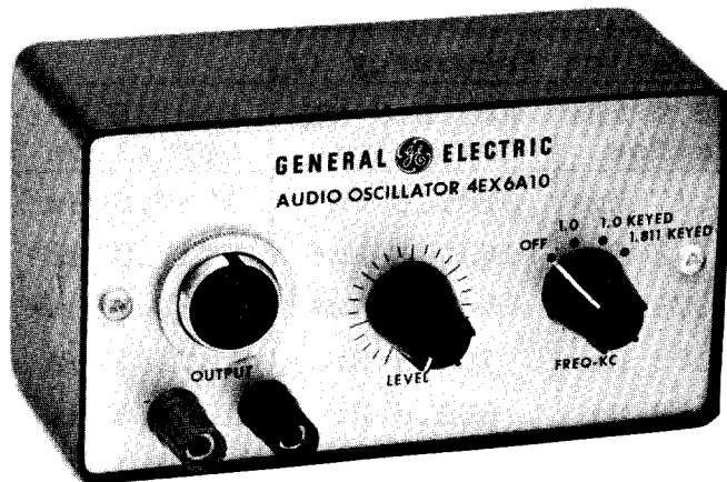
Figure 3 - The 1811-Hz output of Oscillator EX-6-A is very useful in making Bessel null calibrations.
