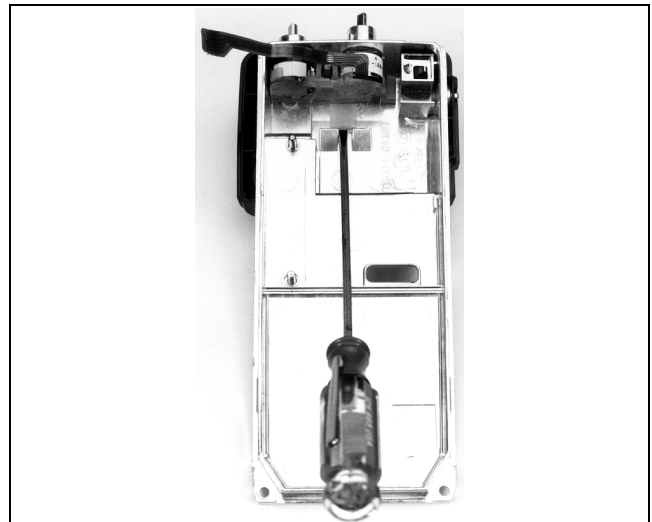
Figure 16 - Removing the Switch Assembly (Pry up on bottom latch)
