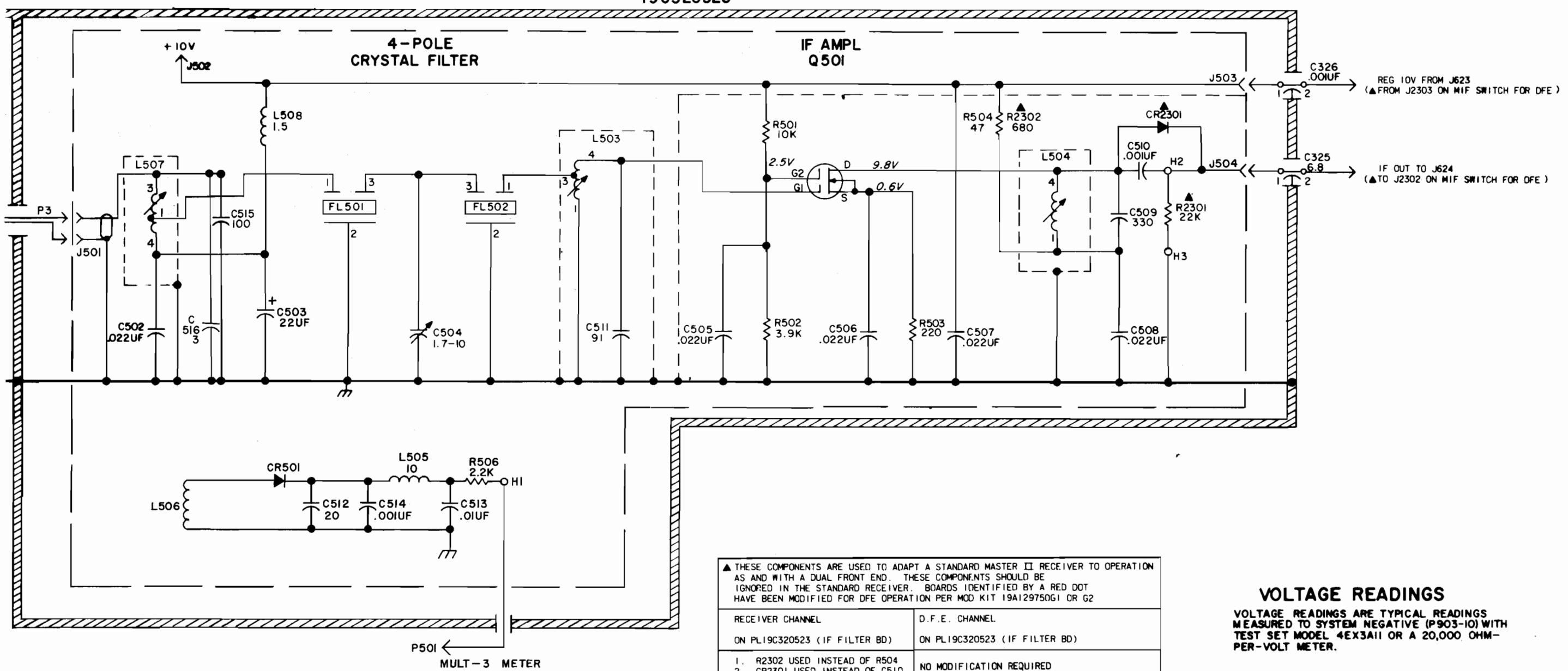
▲ THESE COMPONENTS ARE USED TO ADAPT A STANDARD MASTER II RECEIVER TO OPERATION AS AND WITH A DUAL FRONT END. THESE COMPONENTS SHOULD BE IGNORED IN THE STANDARD RECEIVER. BOARDS IDENTIFIED BY A RED DOT HAVE BEEN MODIFIED FOR DFE OPERATION PER MOD KIT 19A129750G1 OR G2
