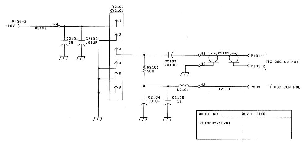
ALL RESISTORS ARE 1/4 WATT UNLESS OTHERWISE SPECIFIED AND RESISTOR VALUES IN OHMS UNLESS FOLLOWED BY K-1000 OHMS OR MEG-1,000,000 OHMS. CAPACITOR VALUES IN PICOFARADS (EQUAL TO MICROMICROFARADS) UNLESS FOLLOWED BY UF-MICROFARADS.
